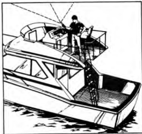
Give Antenna Direct View of Satellites
