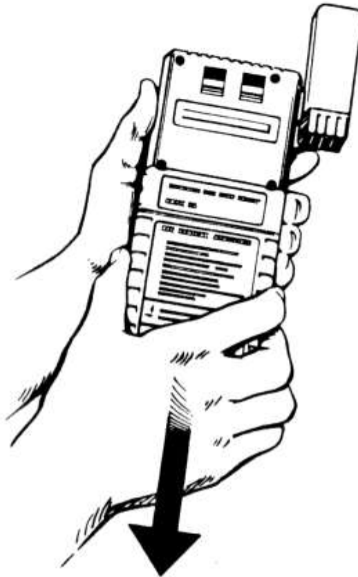
Opening the Battery Door
