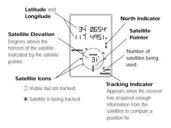
You may sometimes notice that the number of satellites being tracked differs from the number of satellites being displayed graphically. This is due to more than one satellite being tracked in the same general area.
