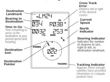
The navigation screens and the position screen are connected to one another in a circular loop. Pressing the  $\boxed{NAV}$  key or using the ARROW pad while viewing one of the position or navigation screens moves you to the next screen in the loop.
