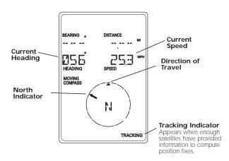
The navigation screens display your speed of travel. For the speed to be displayed, you must be moving at a speed greater than 2 miles per hour.
